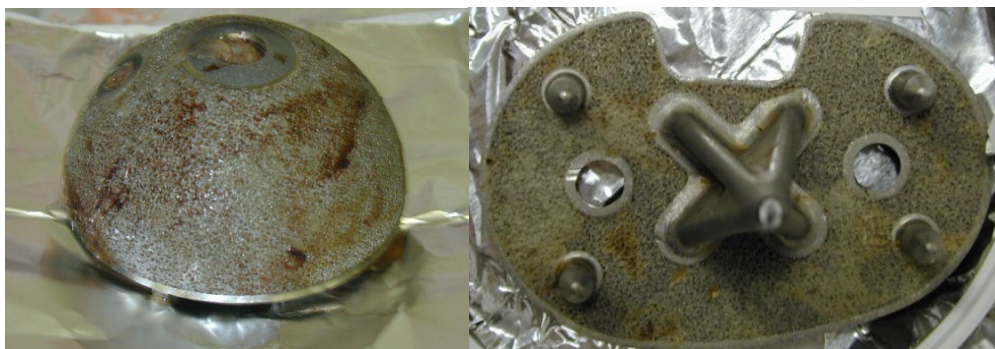
Figure 1: Examples of explanted devices that were removed due to poor fixation.
