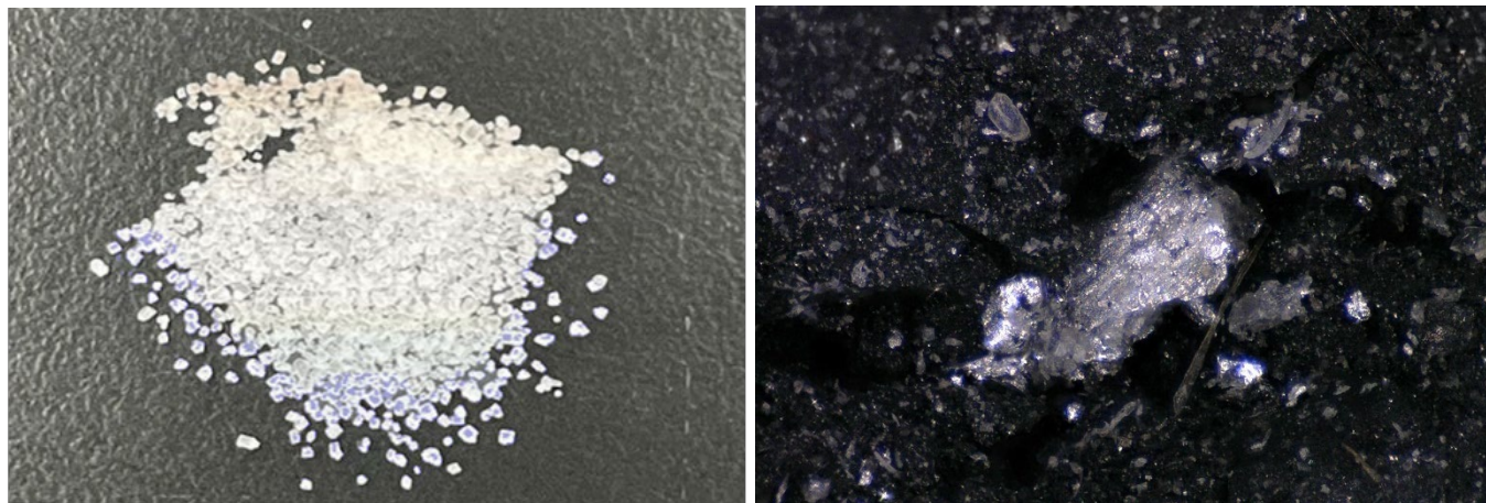
Figure 1: Left: The discoloration on the vial wall was identified as radiant particulates clustered near the rubber septum. Right: Adjacent to the particulate, the rubber septum was torn and discolored.
