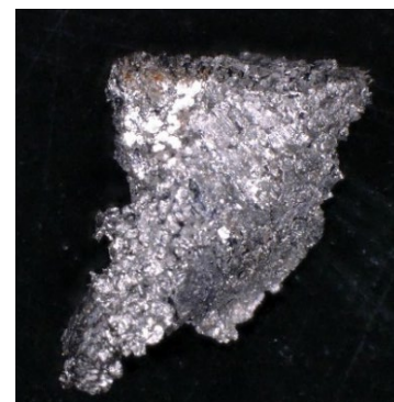
Figure 2: A galvanized steel particle was embedded in the rubber septum near the particulate on the vial wall.
