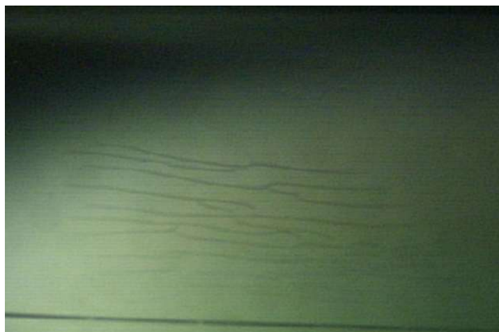
Figure 1: Microcracks forming in PC syringe.
