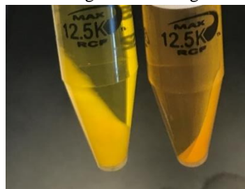
Figure 3: Pellets obtained following extraction of curcuminoids with methanol and centrifugation for the experimental sample (left) and the curcumin control (right).
