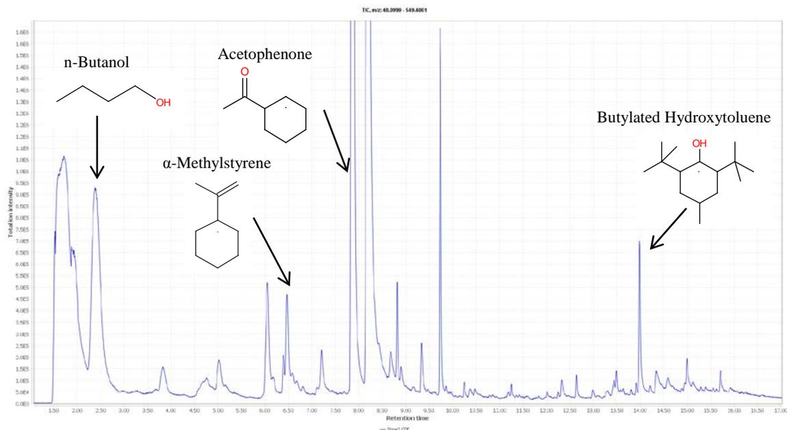
Figure 4: Total ion chromatogram for the Nike sole. A subset of the identified compounds is indicated with their chemical structures.
