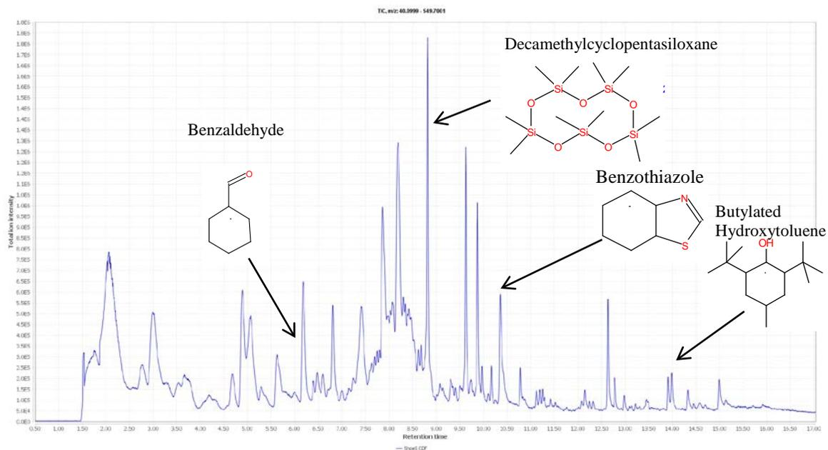
Figure 5: Total ion chromatogram for the Vibram sole. A subset of the identified compounds is indicated with their chemical structures.
