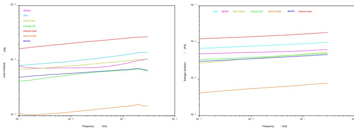
**Figure 3: Loss Modulus (left) and Storage Modulus (right) overlay of shoe samples during frequency sweep from 0.1 Hz to 30 Hz.**
