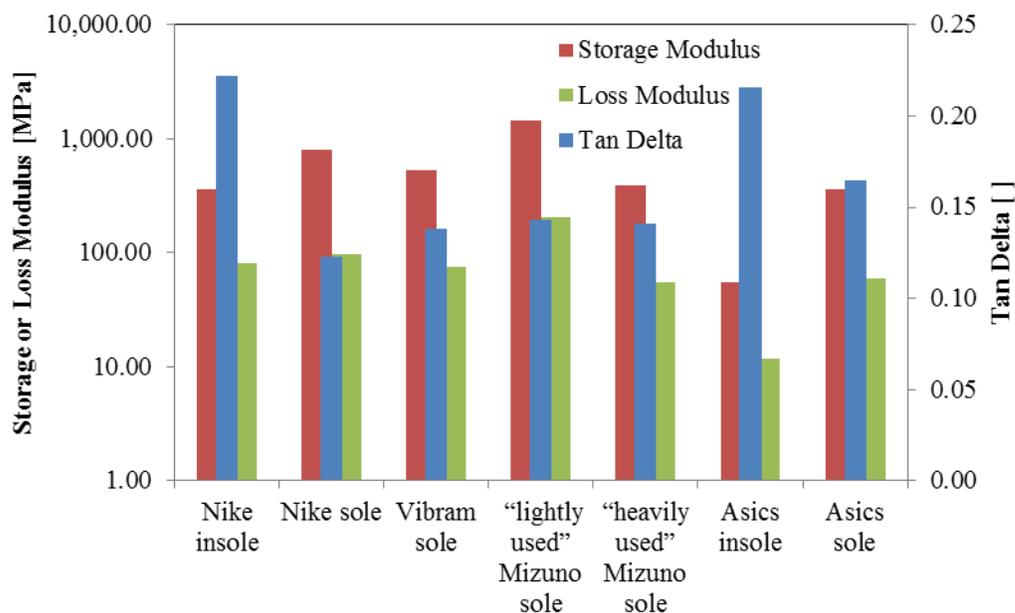
Figure 2: Summary of Storage and Loss Modulus, as well as Tan Delta, at 1 Hz for all shoe samples tested.
