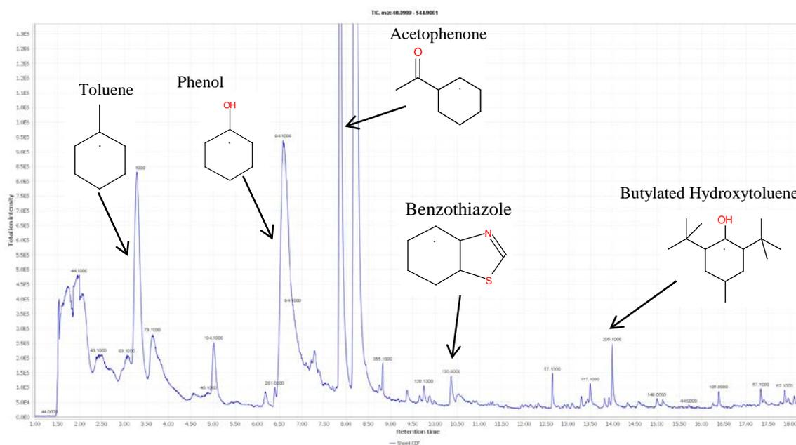
Figure 6: Total ion chromatogram for "lightly used" Mizuno Sole. A subset of the identified compounds is indicated with their chemical structures.
