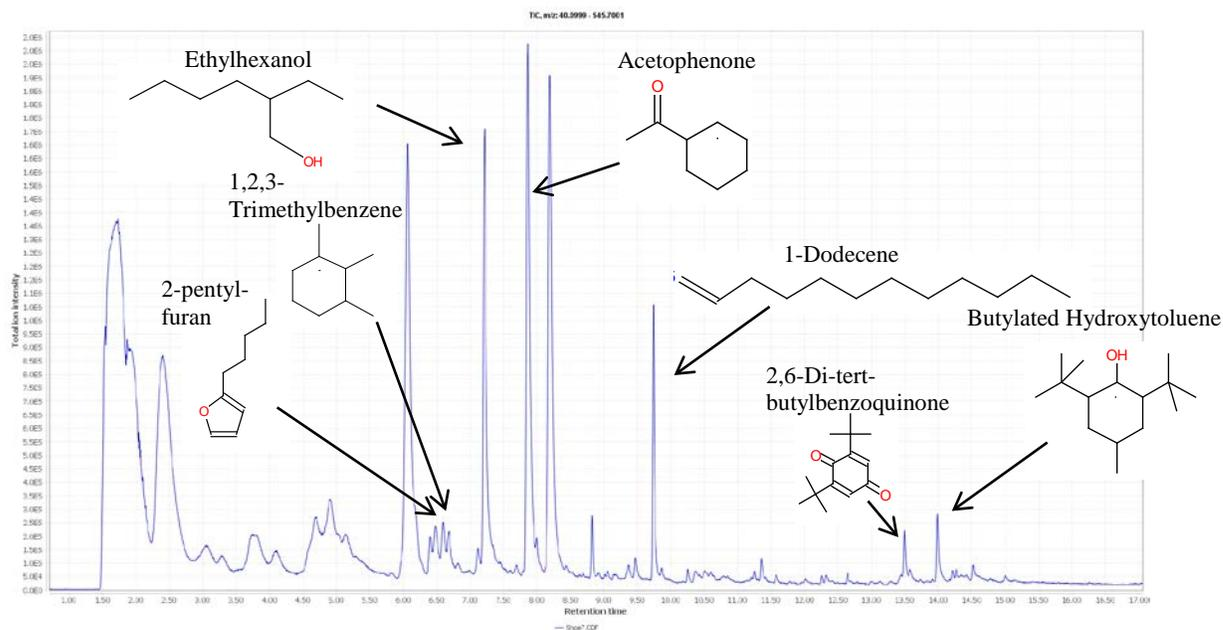
**Figure 7: Total ion chromatogram for Asics sole. A subset of the identified compounds is indicated with their chemical structures.**
