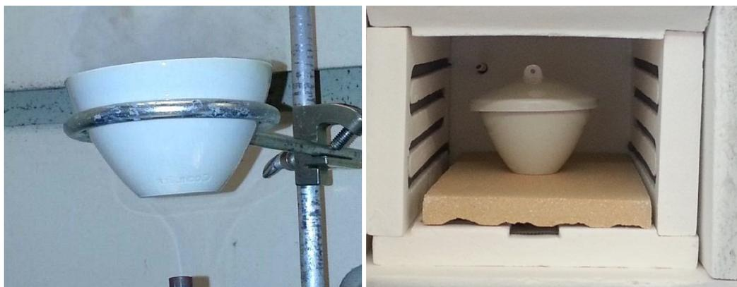
**Figure 1: Crucible undergoing pre-burn with a propane torch to burn off the bulk of the sample (left), followed by incineration in the muffle furnace at 800°C for the complete ashing.**
