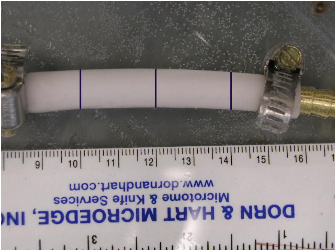
Figure 1: Hydrogel expansion at an internal pressure of 78 mm Hg. Vertical lines indicate the diameter measurement locations. 78 mm Hg.
