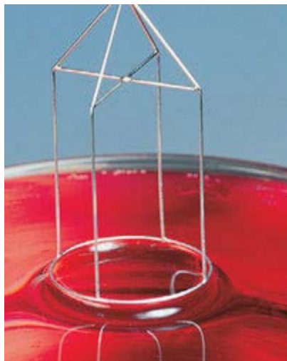
Figure 5: Image of a de Noüy ring at point where meniscus is stretched to almost breaking point.
