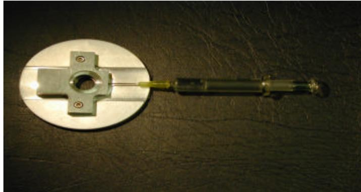
**Figure 2:** Swelling ratio chamber allows microscope access and rapid solvent changes
