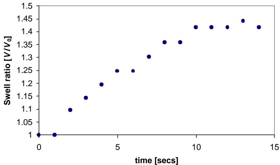
**Figure 5:** Dynamic swell ratio of microspheres as a function of exposure time to solvent.
