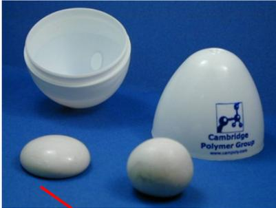
At very long times the material behaves like a liquid spreading out onto a flat surface
