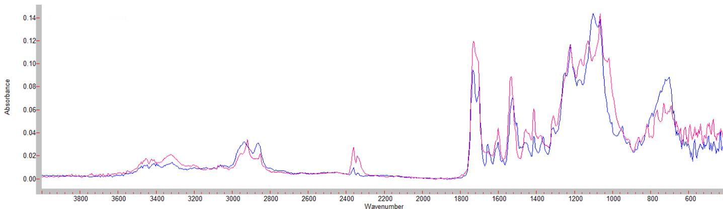
**Figure 1: FTIR spectral comparison of the new (blue) and used (red) basketball material.**
