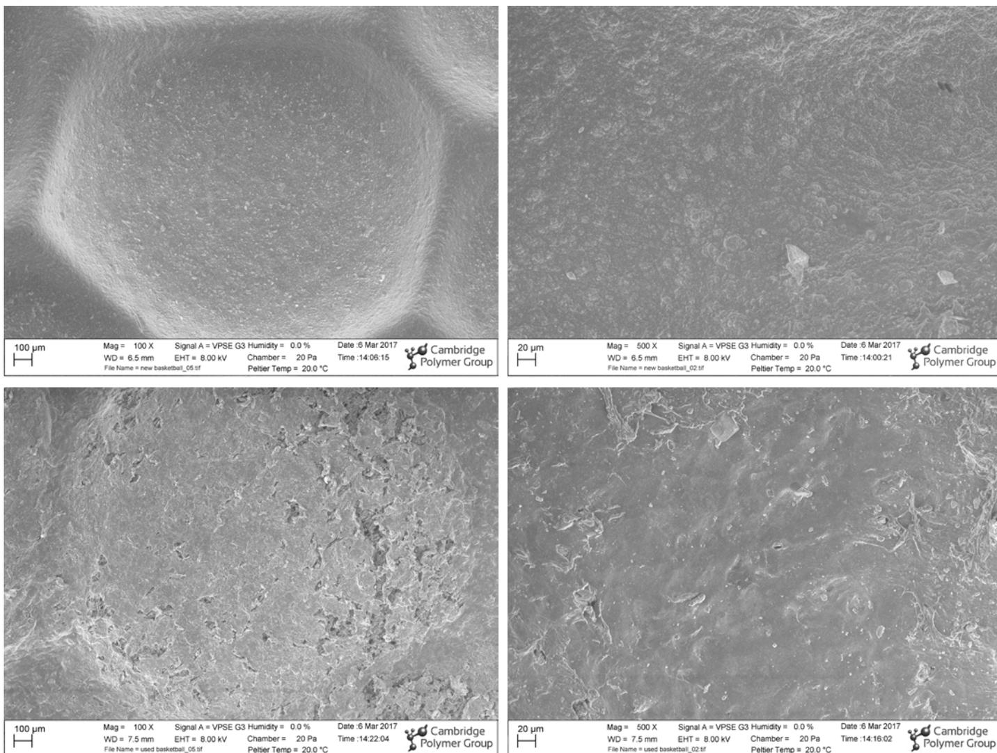
**Figure 2: SEM micrographs of new (top row) and used (bottom row) basketballs revealing the differences in surface morphology between the balls. Micrographs were captured at 100X (left) and 500X (right).**
