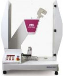
CPG recently purchased a new impact tester, a CEAST 9050 (Instron). With both V-notching and blade notching capabilities, we can perform Izod impact testing on materials in compliance with ASTM D256, as well as impact testing on UHMWPE per ASTM F648. The pneumatic release option on the impact tester allows very reproducible results.
