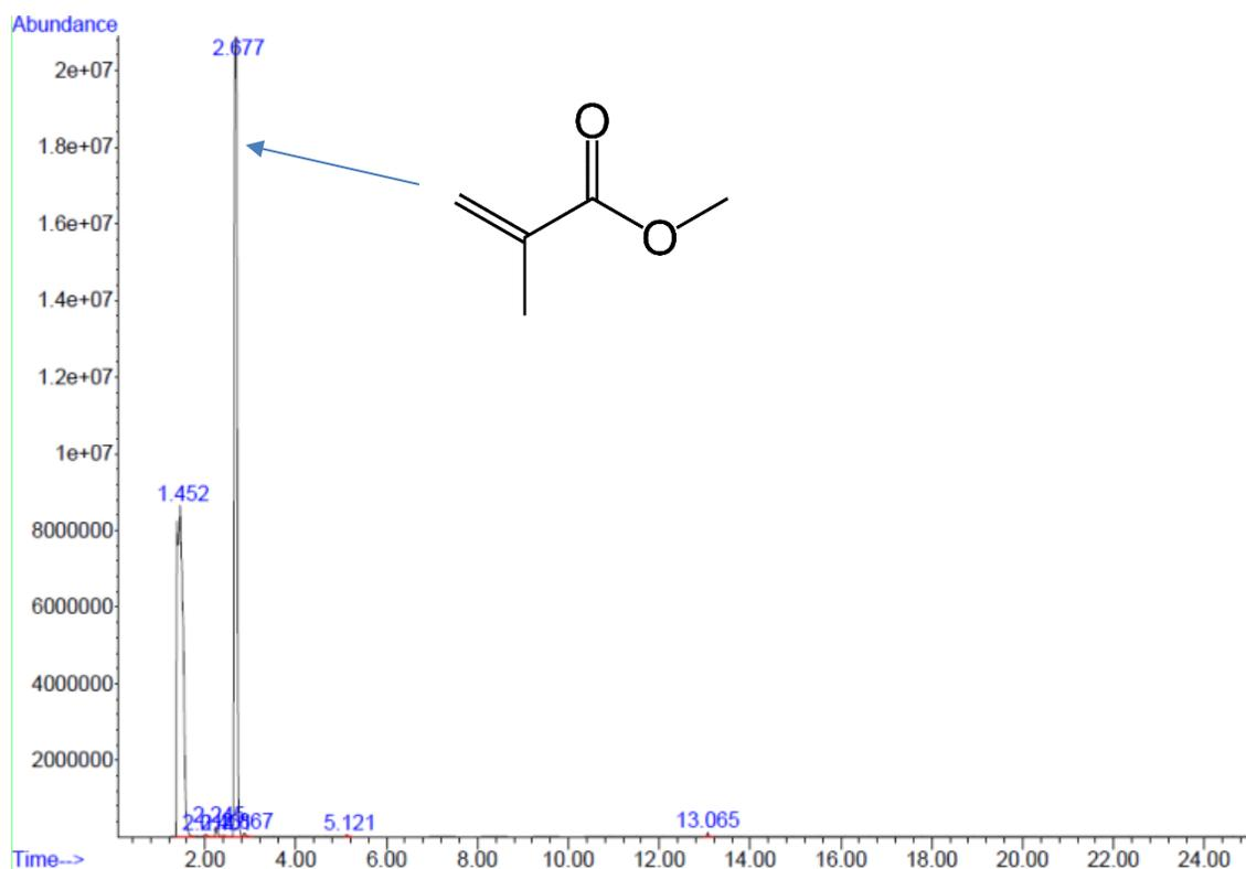
**Figure 1: Total ion chromatogram of PMMA by headspace GC/MS.**
