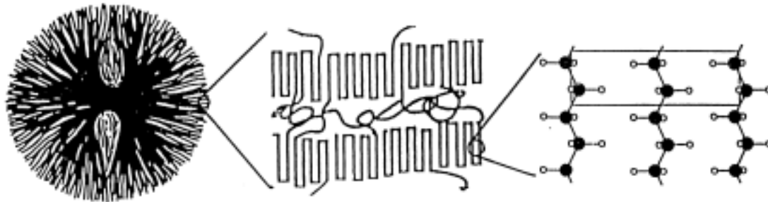
Figure 6: Schematic diagram of a spherulite of polypropylene, showing the large scale structure (left), the chain folding (middle), and the molecular level polymer structure in the folds (right).
