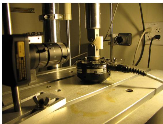
Figure 1: Dual camera automated optical system
