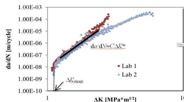
Figure 3: Exemplary  $da/dN$  vs  $DK$  data
