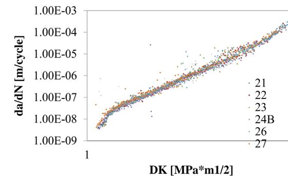
Figure 4:  $da/dN$  vs  $DK$  data for 8 replicate Specimens at Lab 1, showing system repeatability
